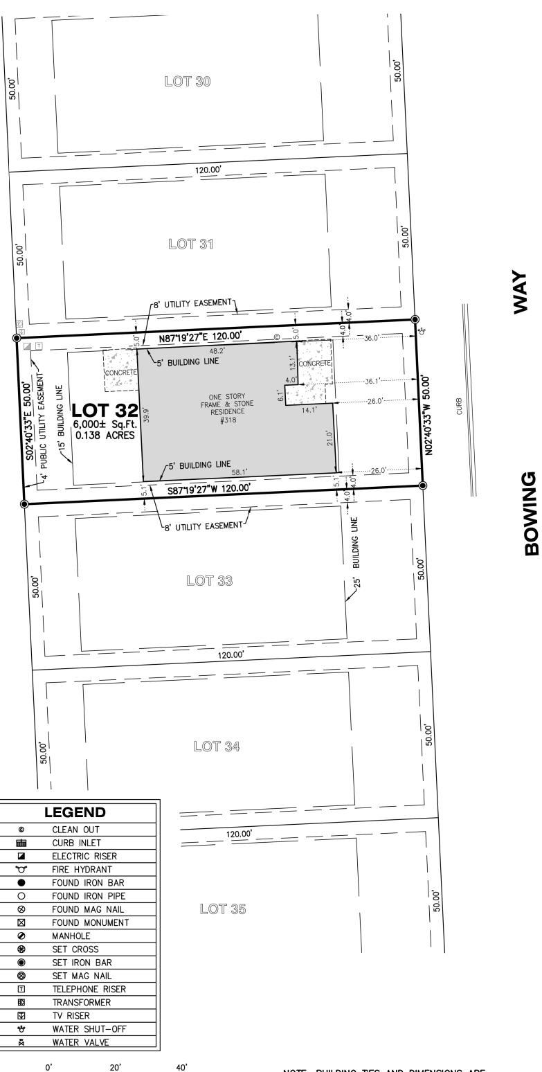
NOTE: BUILDING TIES AND DIMENSIONS ARE MEASURED TO THE FOUNDATION
