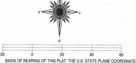
BASIS OF BEARING OF THIS PLAT: THE U.S. STATE PLANE COORDINATE SYSTEM SOUTH ZINE, GRID NORTH NAD 83.
