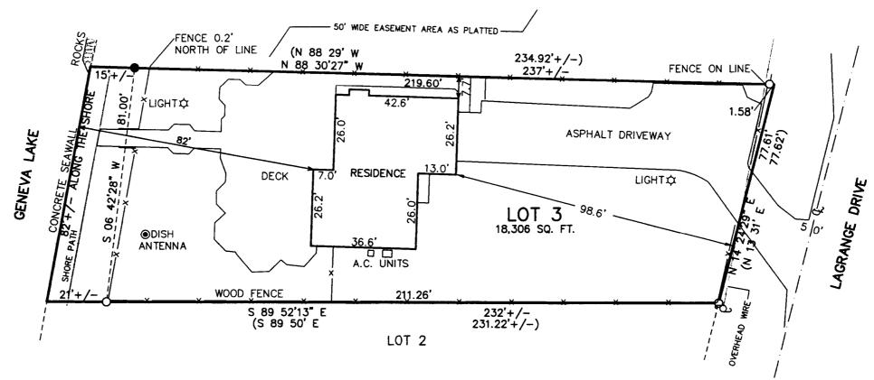
EASEMENTS FOR WATER AND SEWER DOC. NO.'S 498209 AND 563684 RUN WITHIN THE PLATTED ROW FOR LAGRANGE DRIVE.
