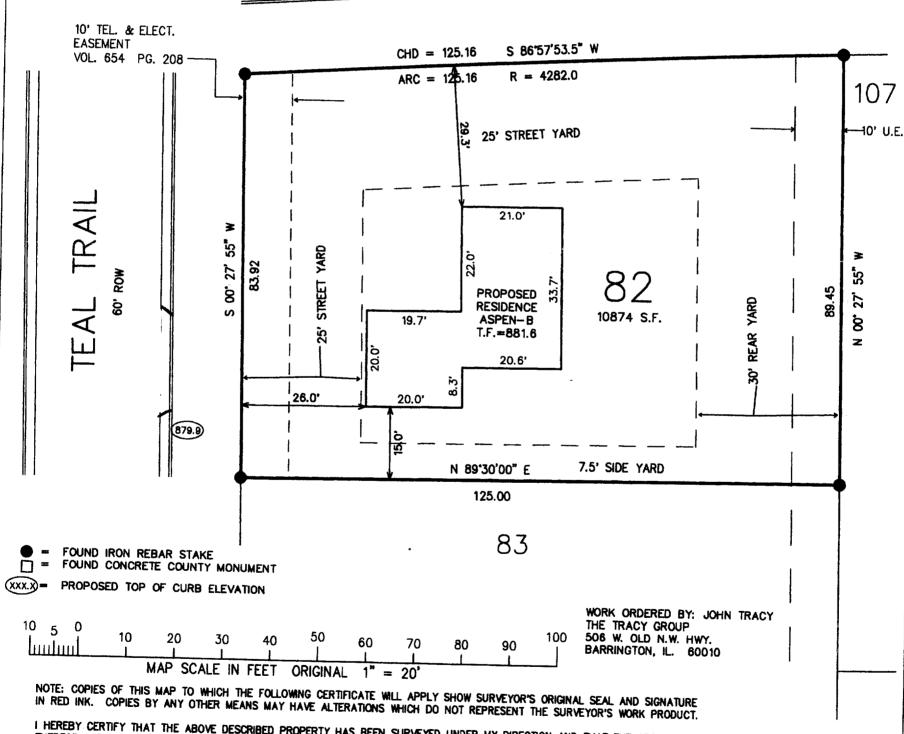
I HEREBY CERTIFY THAT THE ABOVE DESCRIBED PROPERTY HAS BEEN SURVEYED UNDER MY DIRECTION AND THAT THE ABOVE MAP IS A TRUE REPRESENTATION THEREOF AND SHOWS THE SIZE AND LOCATION OF THE PROPERTY, ITS EXTERIOR BOUNDARIES, THE LOCATION OF ALL VISIBLE STRUCTURES, AND DIMENSIONS OF THE USE OF THE PRESENT OWNERS OF THE PROPERTY, AND ALSO THOSE WHO PURCHASE, MORTGAGE, OR GUARANTEE THE TITLE THERETO WITHIN ONE YEAR FROM THE DATE HEREOF.
