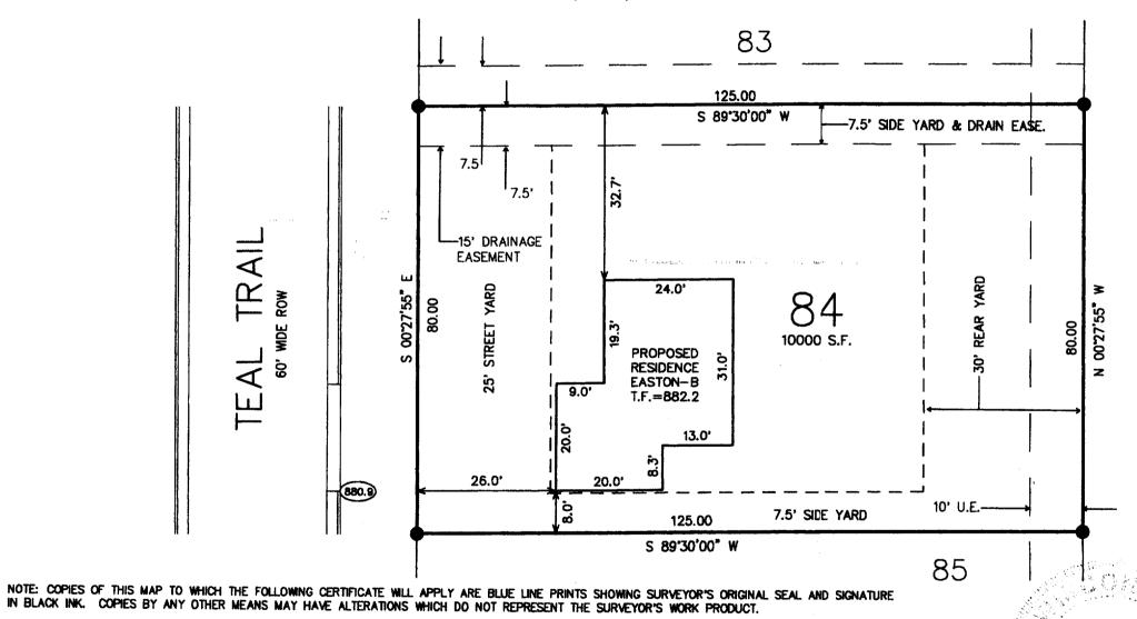
FOUND IRON REBAR STAKE = FOUND CONCRETE COUNTY MONUMENT (XXX.X)= PROPOSED TOP OF CURB ELEVATION
