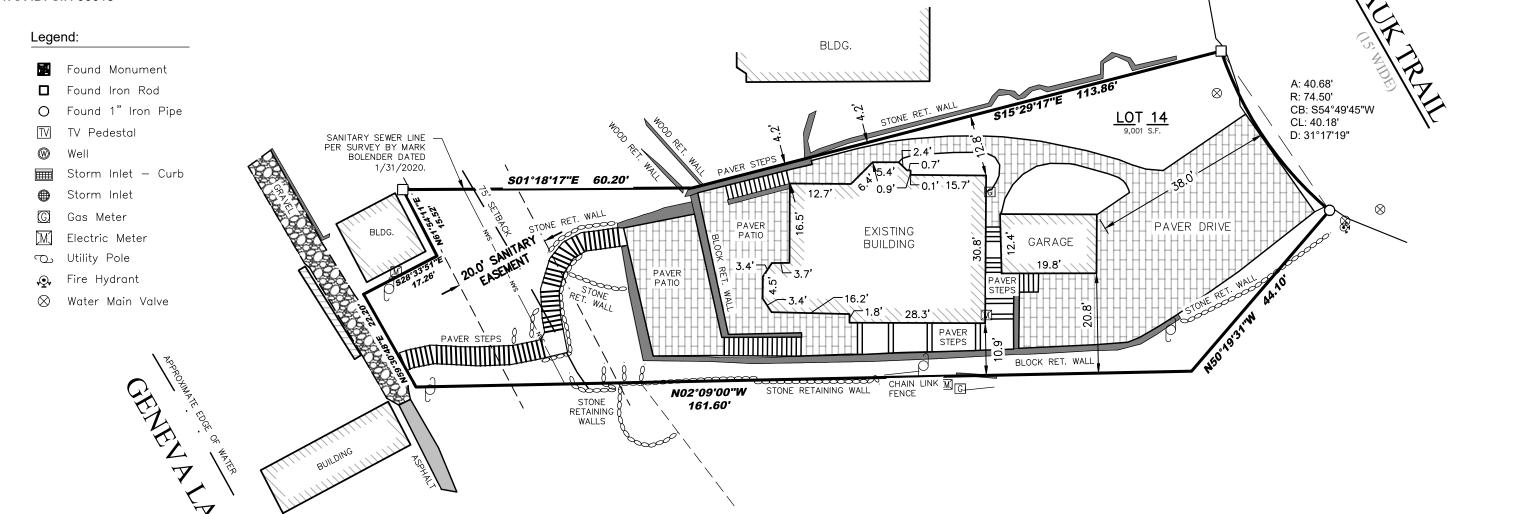
Impervious Area Calculation Area (s.f.) 541 Retaining Walls 1805 Paver Drive Paver Patios 949 662 Steps 1528 Buildings 5486 Total Impervious Lot Area Percent Impervious 60.95%
