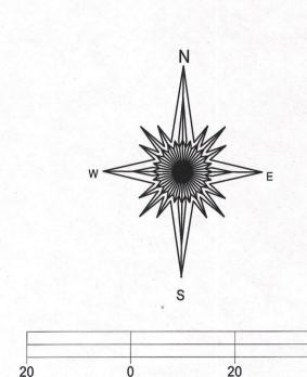
BASIS OF BEARING OF THIS PLAT: THE SUBDIVISION PLAT OF RECORD, THE WEST LINE OF TIMBER TR. WAS ASSUMED TO BEAR N 12°01' W.
