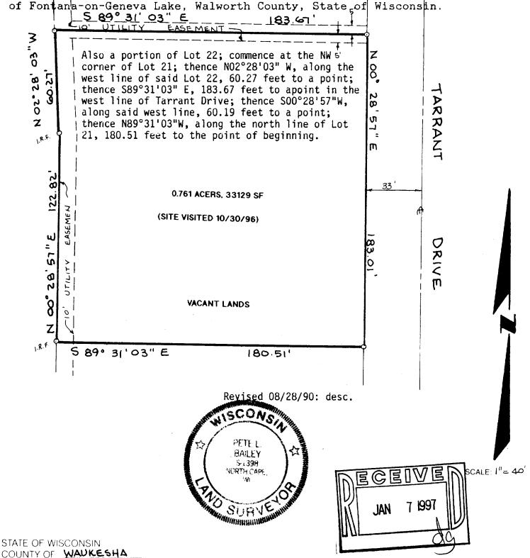
I hereby certify that I have surveyed the above described property and the above map is a true representation thereof and shows the size and location of the property, its exterior boundaries, the location of all visible structures and dimensions of all principle buildings thereon, boundary fences, apparent easements, roadways and visible encroachments, if any.
