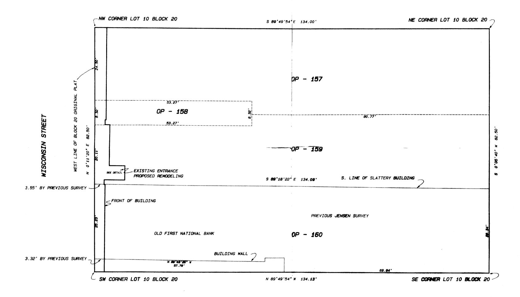
THIS PLAT HAS BEEN PREPARED FROM EXISTING SURVEYS OF RECORD AND LEGAL DESCRIPTIONS WHICH HAVE BEEN PROVIDED BY THE OWNERS. THE PURPOSE OF THIS PLAT IS TO OBTAIN THE NECESSARY PERMITS FOR CONSTRUCTION OF A WHEEL CHAIR RAMP IN ORDER TO COMPLY WITH THE DISABLED AMERICANS ACT. THE REMODELING WILL OCCUR AND BE LIMITED TO THE EXISTING ENTRANCE FOR THE GODFREY, NESHEK, WORTH AND LIEBSLE, S.C. LAW FIRM BUILDING.
