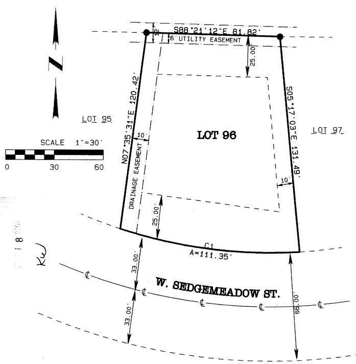
NOTE: FRONT CORNERS TO BE SET UPON CONSTRUCTION OF ROAD AND FINAL GRADING.
