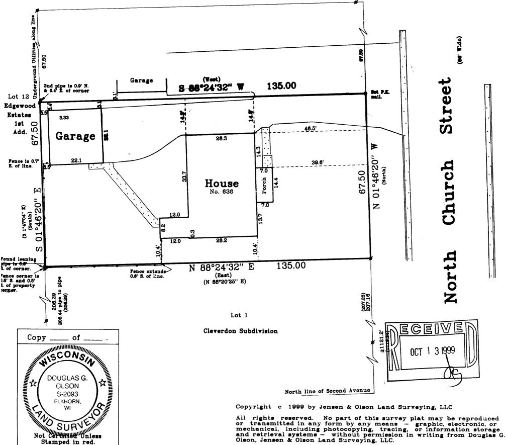
Note: This survey plat is not certified unless signed and sealed in red link.
