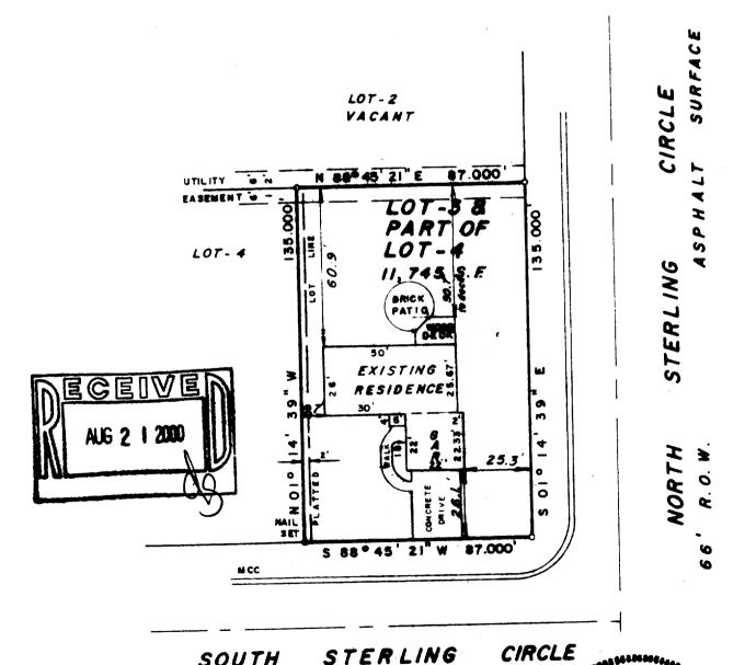
ASPHALT R. O. W. STATE OF WISCONSIN COUNTY OF WAUKESHA JAHNIC inke a jahnke associates inc., do hereby certify that we have made to THE ABOVE PLAT OF SURVEY IS TRUE AND CORRECT REPRESENTATION THEREOF.
