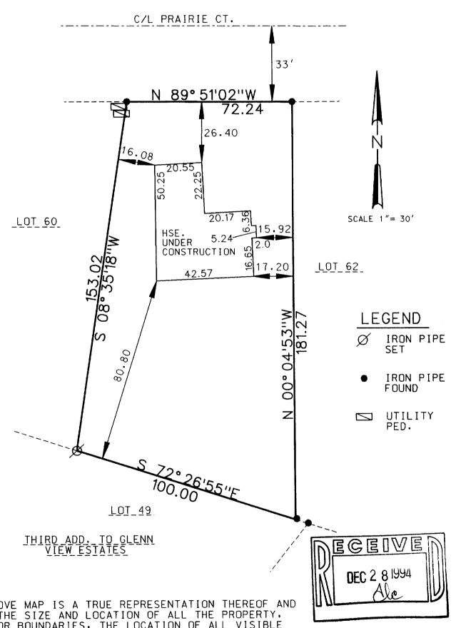
THE ABOVE MAP IS A TRUE REPRESENTATION THEREOF AND SHOWS THE SIZE AND LOCATION OF ALL THE PROPERTY, EXTERIOR BOUNDARIES, THE LOCATION OF ALL VISIBLE BOUNDARY FENCES, APPARENT EASEMENTS, ROADWAYS AND VISIBLE ENCROACHMENTS, IF ANY.
