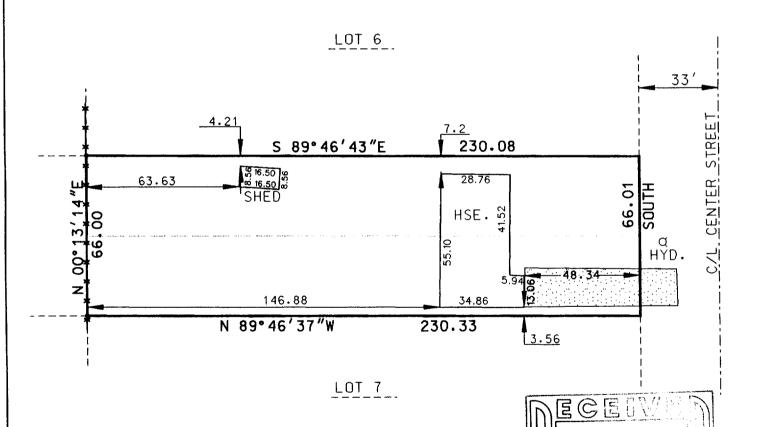
THE ABOVE MAP IS A TRUE REPRESENTATION THEREOF AND SHOWS THE SIZE AND LOCATION OF ALL THE PROPERTY, EXTERIOR BOUNDARIES, THE LOCATION OF ALL VISIBLE BOUNDARY FENCES, APPARENT EASEMENTS, ROADWAYS AND VISIBLE ENCROACHMENTS, IF ANY.
