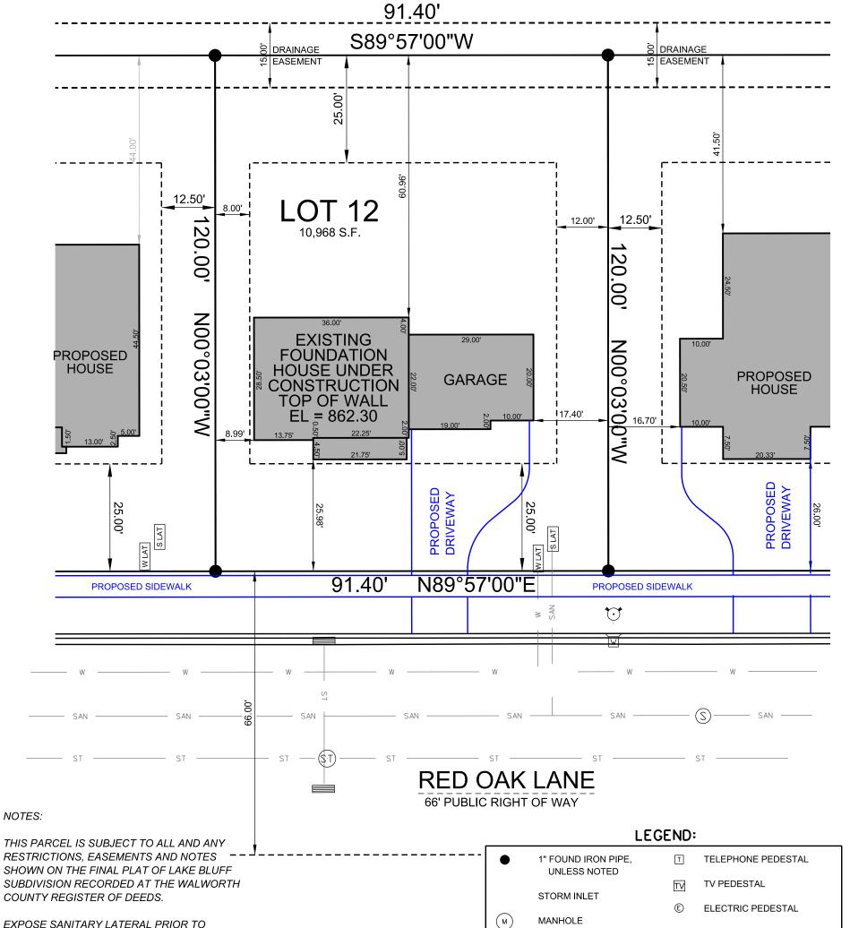
EXPOSE SANITARY LATERAL PRIOR TO CONSTRUCTION TO VERIFY GRAVITY FLOW TO BASEMENT.
