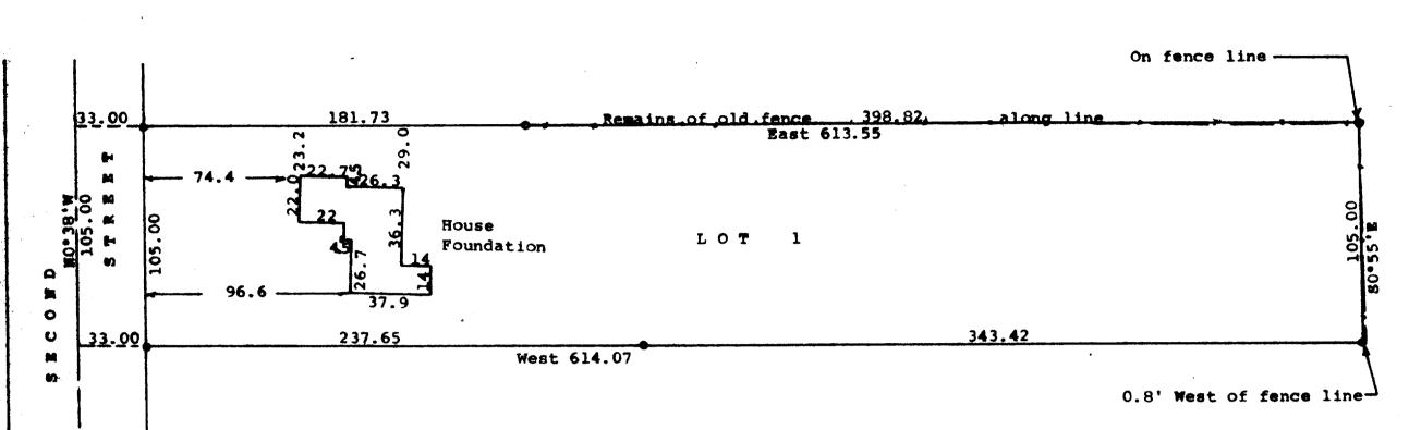
Scale - 1" = 50'•= 1" Iron Pipe Found o = 3" Iron Pipe Found -- = Fence Line Bearings are those shown on the recorded plat of CSM No. 566 Survey ordered by: Jeff Goff 300 Bradley Avenue Delavan, WI 53115
