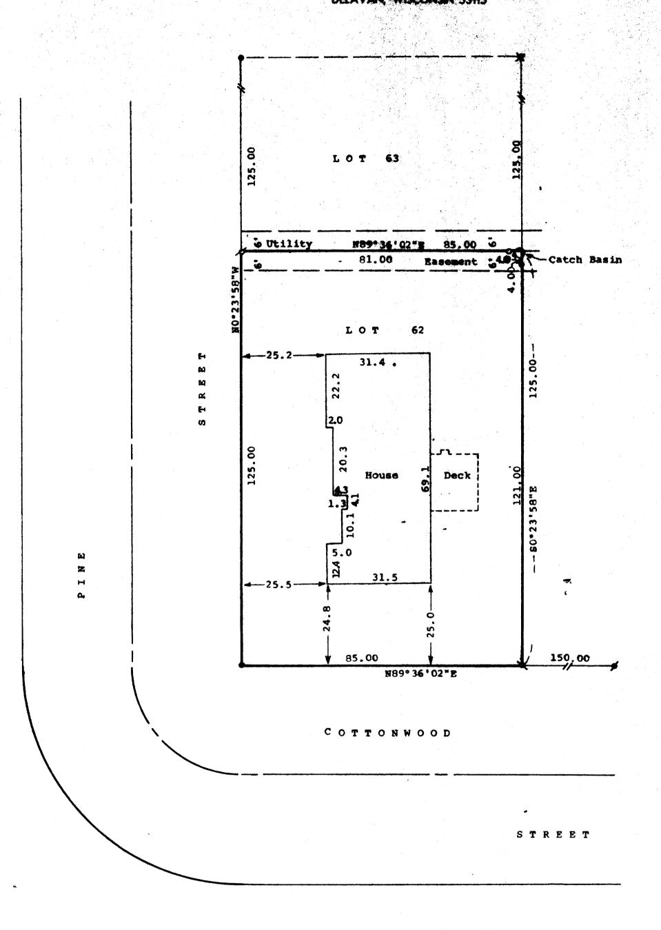
Scale - 1" = 20'• =1 3/16" Dia. Iron Bar Found m = 5/8" Dia. Iron Bar Found & Reset # = 3/4" Dia. Iron Pipe Found o = 3/4"x24" Iron Pipe Set X = 1" Iron Pipe Found Bearings are those of record.
