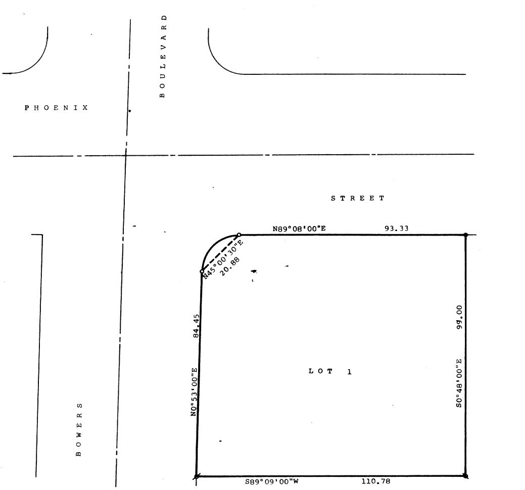
Scale - 1" = 20'• = Broken Concrete Monument Found and Reset with 1"x24" Iron Pipe o = 2" Dia. Iron Pipe Found # = 1 Dia. Iron Pipe Found a = 3/4" Dia. Iron Pipe Found
