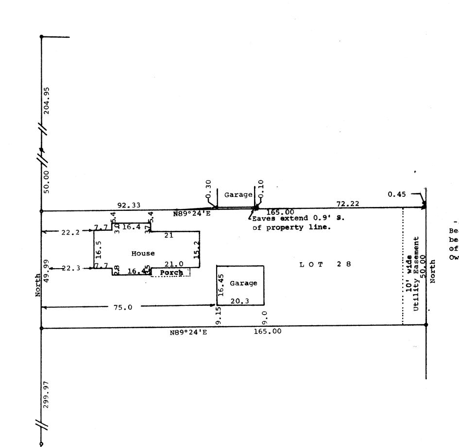
Scale - 1" = 20'• = Concrete Monument Found ≠= 1½" Iron Pipe Found w= 1" Iron Pipe Found o = 3/4" Iron Pipe Found - = Fence Line Bearings referenced to the assumed bearing of North along the east line of Bradley Avenue Owners: Bradway & Charlotte Liddle
