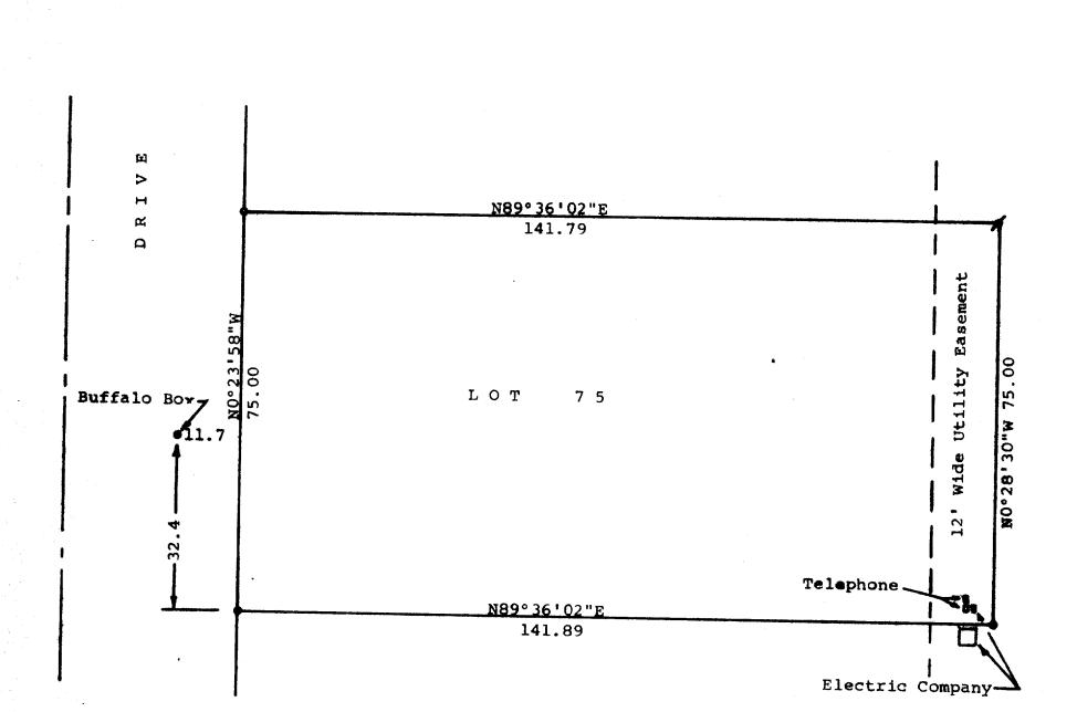
Scale - 1" = 20!e = 1" Iron Pipe Found ≠ = 1" Iron Pipe Found Bent. Pulled, straightened and reset Bearings shown are those of record Survey ordered by: Keefe Real Estate Inc. Better Homes & Gardens 302 East Walworth Avenue Delavan, WI 53115
