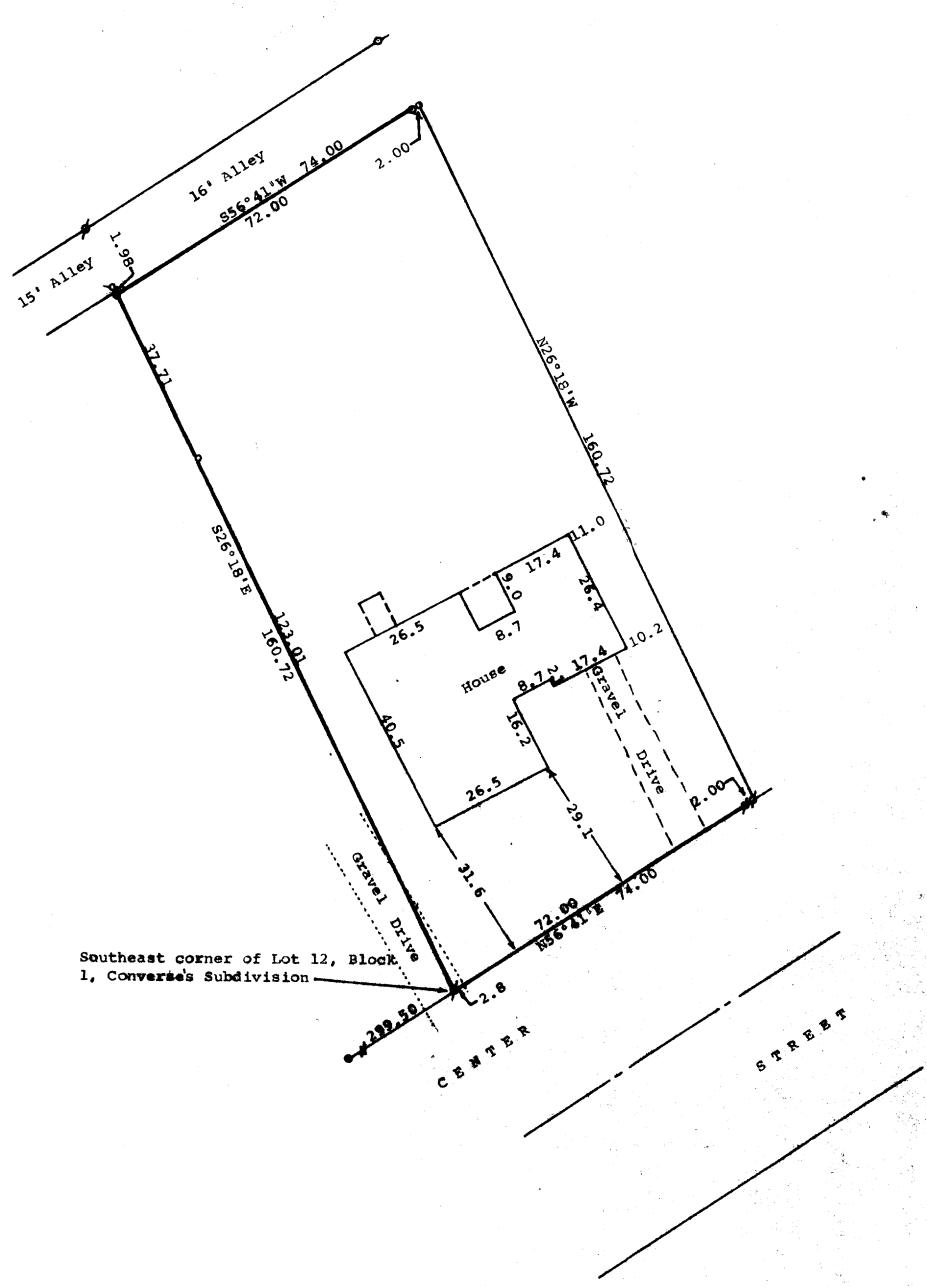
Scale - 1" = 20' • = Concrete Monument Found h= 1" Dia. Iron Pipe Found 1" Down and reset with a 4"x24" Iron Pipe #= 1" Dia. Iron Pipe Found 1' Down And reset at surface 0= 1" Dia. Iron Pipe Found \$\delta = 3/4" Dia, Iron Pipe Found p= '5" Dia. Rod Found
