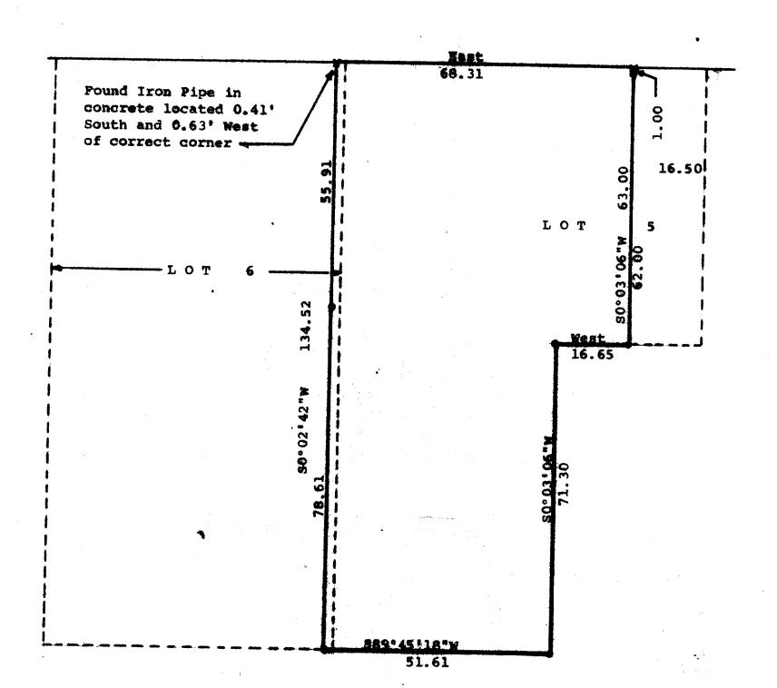
Scale -1" = 20"•= Iron Pipe Found X= Cross in Concrete •= Iron Pipe in Concrete
