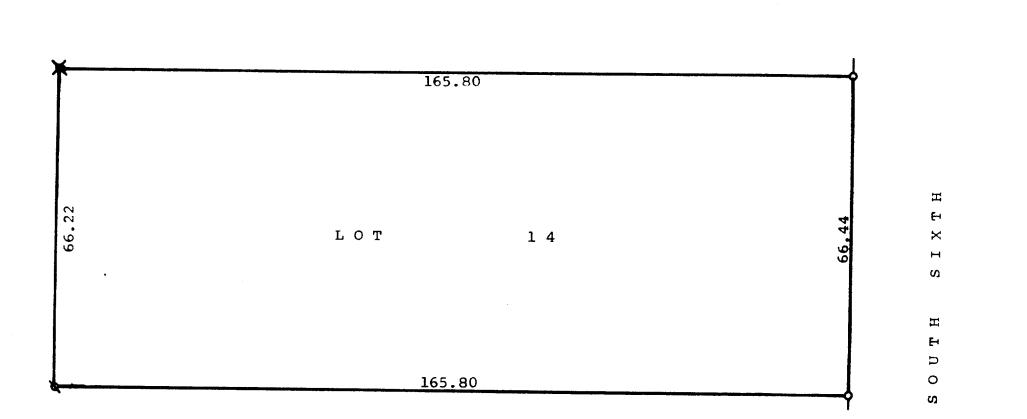
Scale - 1" = 20'and Reset 0 = Iron Pipe Set **Q** = Iron Pipe Found
