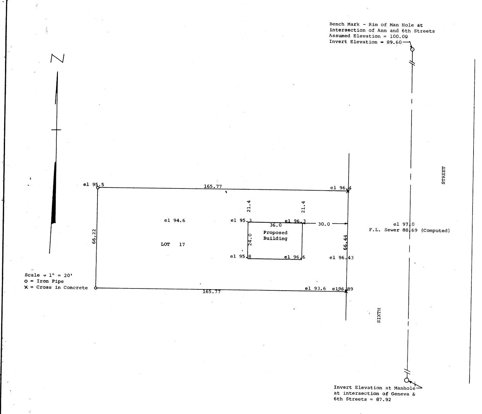
Plat of survey of Lot 17, Block 4 of Passage, Aram & Downie Addition to the City of Delavan, Walworth County, Wisconsin, showing the location of a proposed building to be built on said lot and elevations on the ground at various points.
