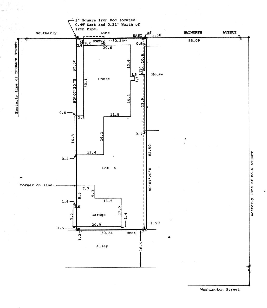
Scale - 1" = 10•= Concrete Monument Found == 1" Square Iron Rod Found  $\phi = 3/4$ " Dia. Iron Pipe Found 0 = 3/4"x24" Iron Pipe Set
