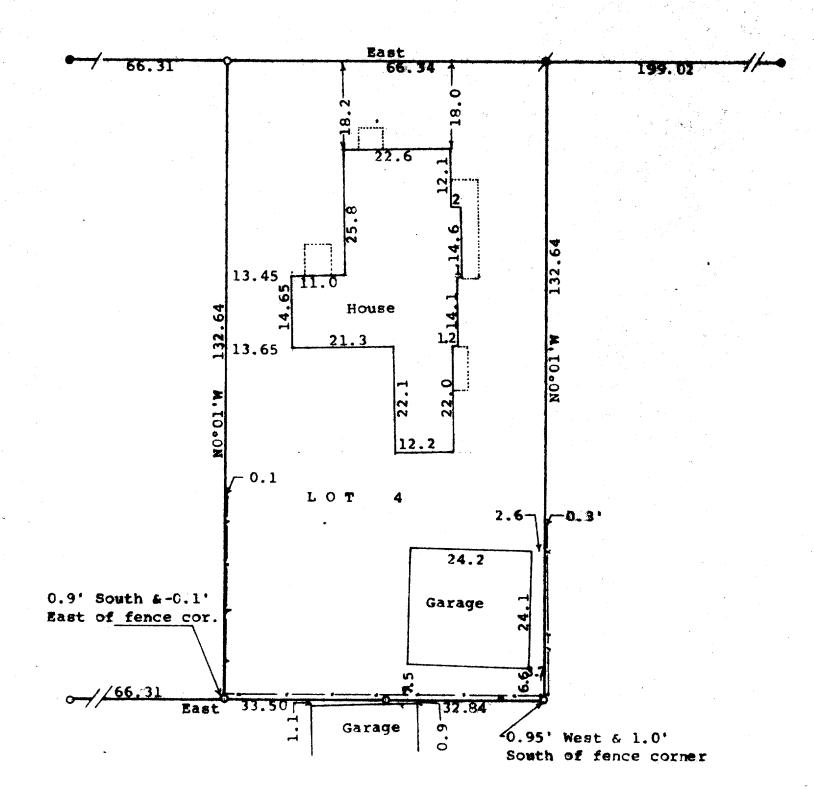
Scale - 1" = 20'• = concrete Monument Found # cross cut on top of conc. monument found o = 3/4" Iron Pipe Found 0= 3/4" X 24" Iron Pipe Set Bearings referenced to the south line of Wisconsin Street with the assumed bearing of East Survey ordered by: Joan Dunham 1913 Swan Creek Delavan, WI 53115
