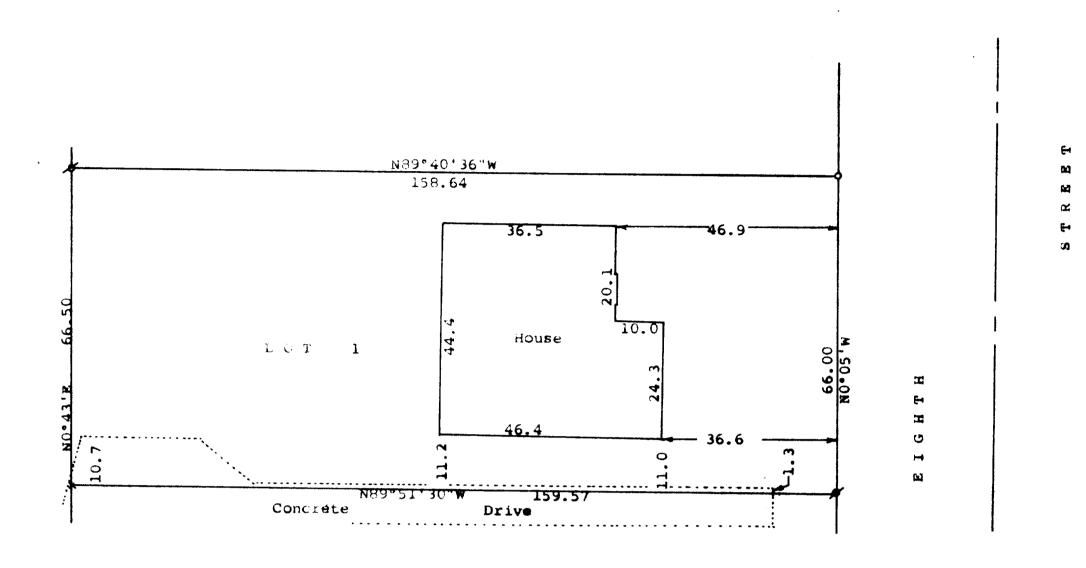
Scale - 1" = 20' X = Cross cut in concrete found  $\beta = 3/4$ " Iron Pipe Found o = 1" Iron Pipe Found Bearings referenced to the previously assumed bearing of NO 05'W along the west line of Eighth Street Survey ordered by: Ron Deschner N. Shore Drive Delavan, WI 53115
