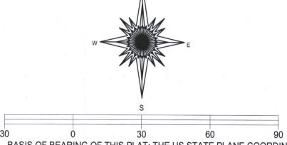
BASIS OF BEARING OF THIS PLAT: THE US STATE PLANE COORDINATE SYSTEM SOUTH ZONE NAD 83 (2011) WISCORS.
