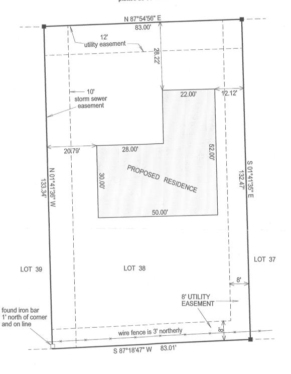
BASIS OF BEARING OF THIS PLAT: THE WEST LINE OF THE NE 1/4 OF SECTION 27-2-15 WAS ASSUMED TO BEAR S1°41'35"E AS SHOWN ON THE RECORD PLAT OF THE PONDS OF DARIEN.
