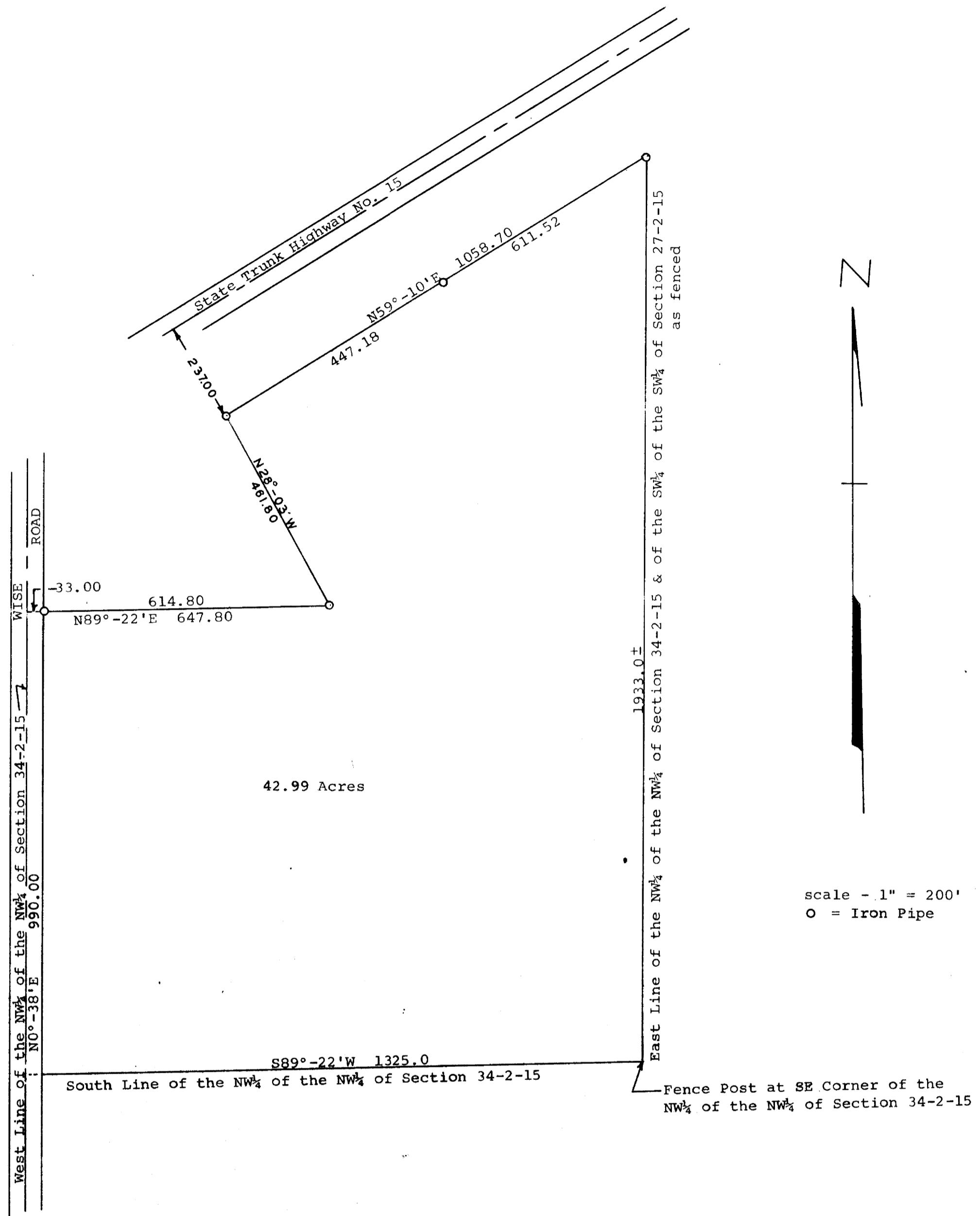
Plat of survey of a parcel of land located in the NW $\frac{1}{4}$  of the NW $\frac{1}{4}$  of Section 34-2-15 & in the SW $\frac{1}{4}$  of the SW $\frac{1}{4}$  of Section 27-2-15 all in T2 N, R 15 E, and part in the Village of Darien, Walworth County, Wisconsin.
