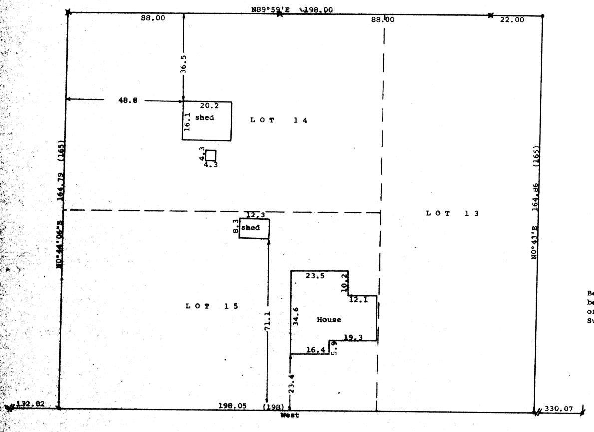
Scale - 1" = 20p = 3/4" Iron Pipe Found M= 1" Iron Pipe Found X= 14" Iron Pipe Found •= 3/4" X 2'\* Iron Pipe Set • = 11 " Iron Pipe Set Bearings referenced to the assumed bearing of West along the north line of Madison Street Survey ordered by: Ken Danielson Realtor
