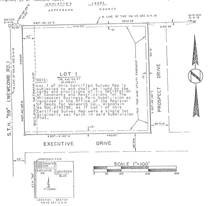
Bearings are referenced to the north line of the NW 1/4 of Sec. 3, T4N, R15E as N  $89^{\circ}$ -59'-23" E.
