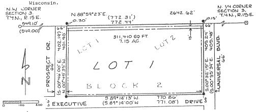
Bearings referenced to the north line of Section 3, assumed N88°59'23"E.
