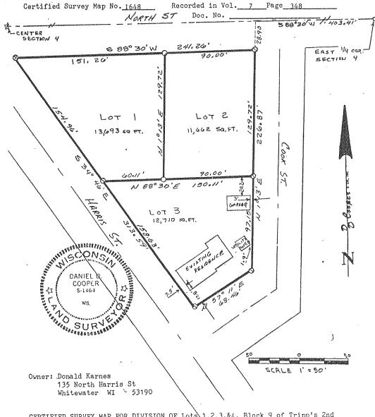
CERTIFIED SURVEY MAP FOR DIVISION OF Lots 1,2,3,&4, Block 9 of Tripp's 2nd Addition to the City of Whitewater, being located in the SE 1/4 of Section 4, T4N, R15E, Walworth County, Wisconsin.
