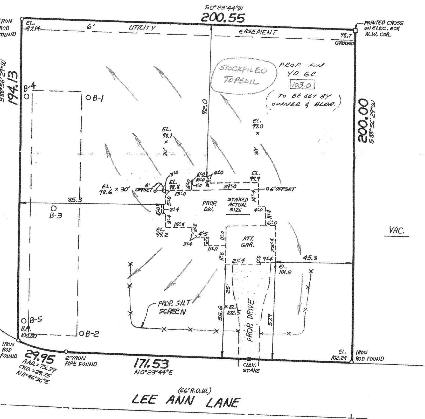
Proposed finished yard. 1st floor or top of foundation grade shown on this drawing is a suggested grade and should be verified by the owner and/or the builder.
