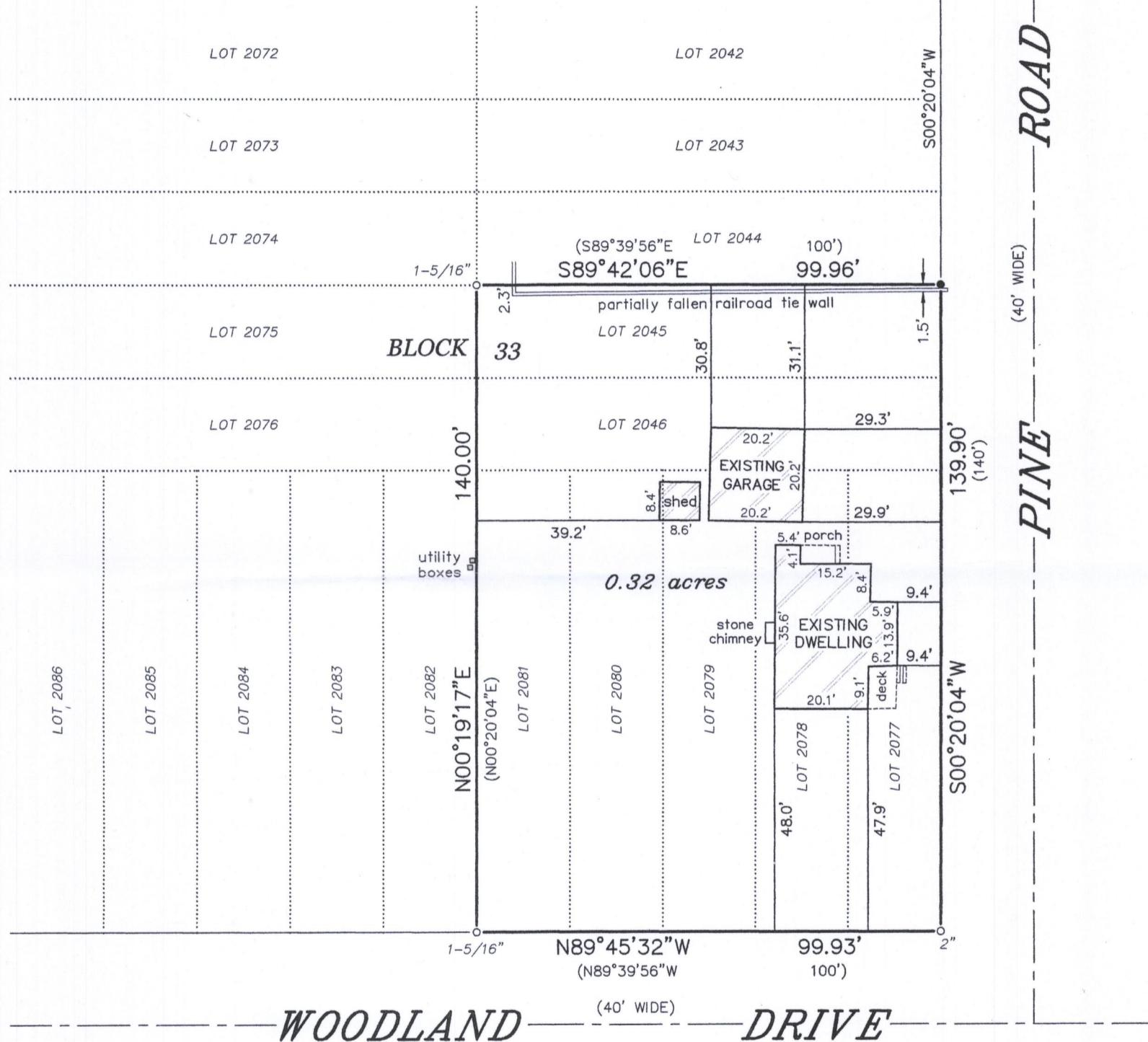
NOTE: RAILROAD TIE RETAINING WALL NEAR THE NORTH PROPERTY LINE LEANS TO THE SOUTH AND APPEARS TO BE FALLEN DOWN IN SPOTS. SNOW COVER MADE IT VERY DIFFICULT TO IDENTIFY THE ORIGINAL LOCATION OF THE WALL. TIES AS DEPICTED HEREON ARE TO THE SOUTH SIDE OF THE WALL AS IT CURRENTLY EXISTS. ALSO, DRIVEWAY WAS SNOW COVERED AND NOT LOCATED AS PART OF THIS SURVEY.
