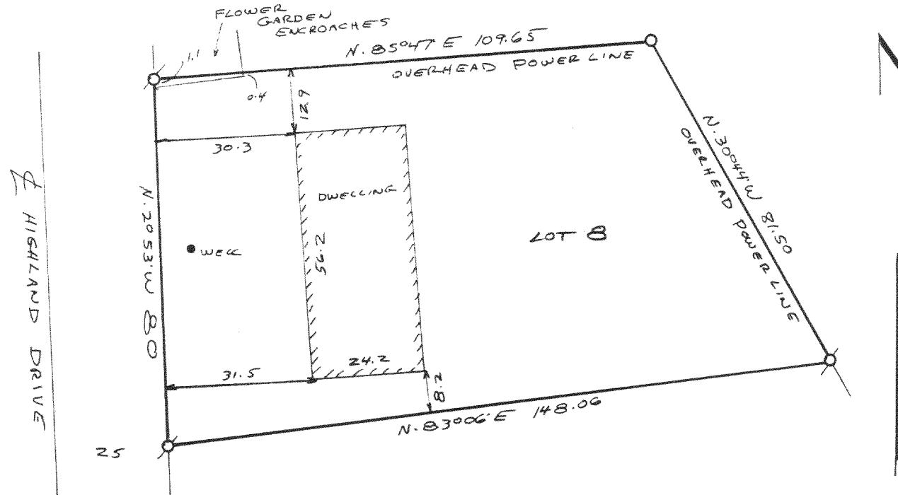
I have surveyed the above-described property, and the map hereon is a true representation thereof and shows the size and location of the property, its exterior boundaries, the location and dimensions of all visible structures thereon, fences, apparent easements and roadways and visible encroachments, if any.
