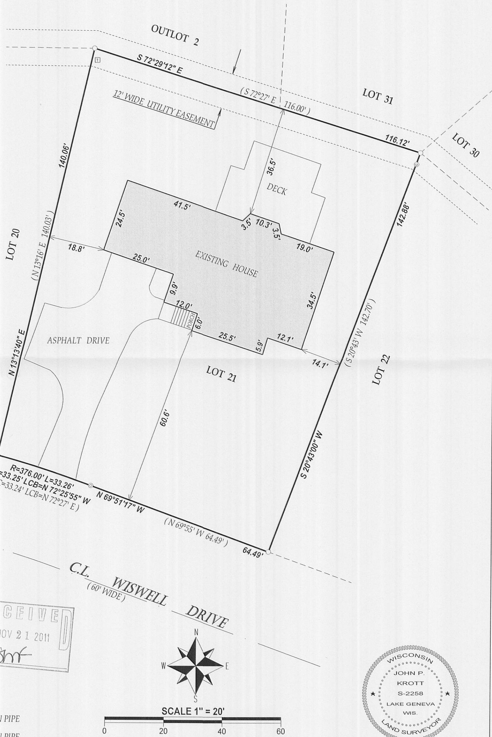
I have surveyed the above-described property and the above map is a true representation thereof and shows the size and location of the property, its exterior boundaries, the location and dimensions of all structures thereon, fences apparent easements and roadways and visible encroachments, if any.
