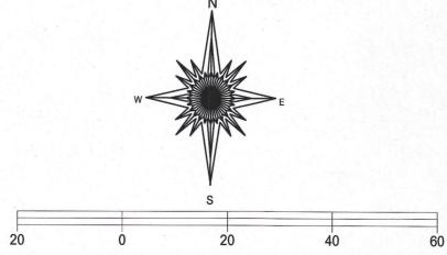
B ASIS OF BEARING OF THIS PLAT: THE WISCONSIN STATE PLANE COORDINATE SYSTEM, SOUTH ZONE, GRID NORTH NAD 83. (WISCORS)
